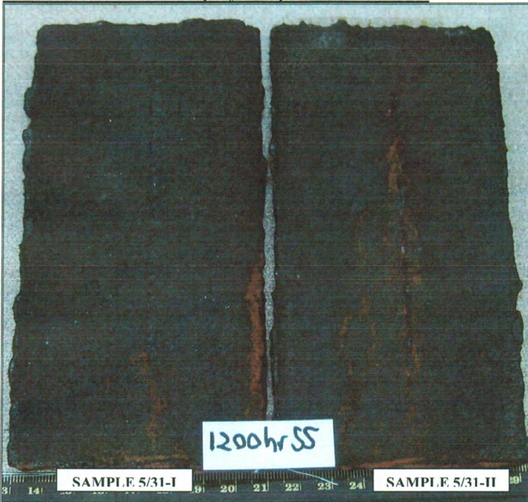
Figure 1: Photograph illustrating specimens after 1200 hours of salt spray exposure.
